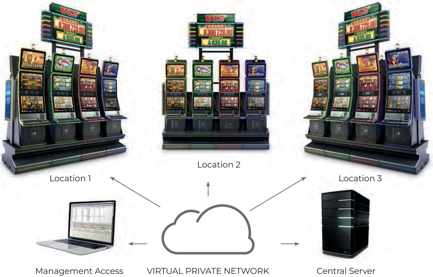
EGT's **Global Solution VLT** is a server-based system that comprises two main components – **Central Server** and **Locations**, with an unlimited number of locations that can be connected to the Central Server.
